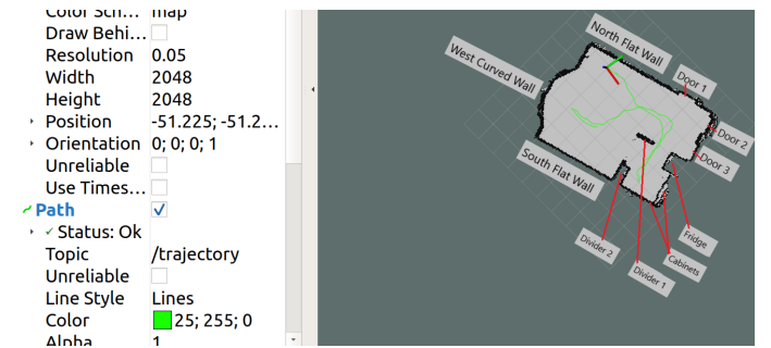
Fig. 12. Scanning result using HectorSLAM.
