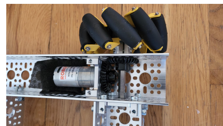
Fig. 5. Close up of the connection between the motor and the mecanum wheel using miter gears and custom designed parts.
